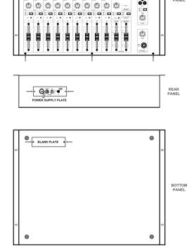
4. Pull out the AC Mains cord attached to the Power Supply Plate through the opening on the Bottom Panel. Now fix the Power Supply Plate on the Bottom Panel using the mounting screws (2 Nos.).
